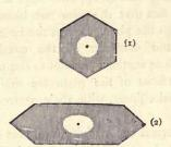
cut (1) perpendicular, (2) parallel, to the axis of the hexagonal prism; along which the conductivity is the greatest. If the substance (as in this case) be homogeneous, the thermal capacity is the same at all points, and thus the results of this experiment are conclusive as to the different conductivities in different directions. By measuring the ratio of the axes of this ellipse and observing their directions, in slices cut with various orientations, we can
